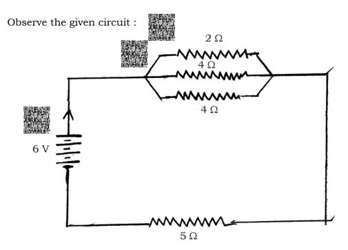
Calculate the total resistance in the circuit and the total current flowing in the circuit.
